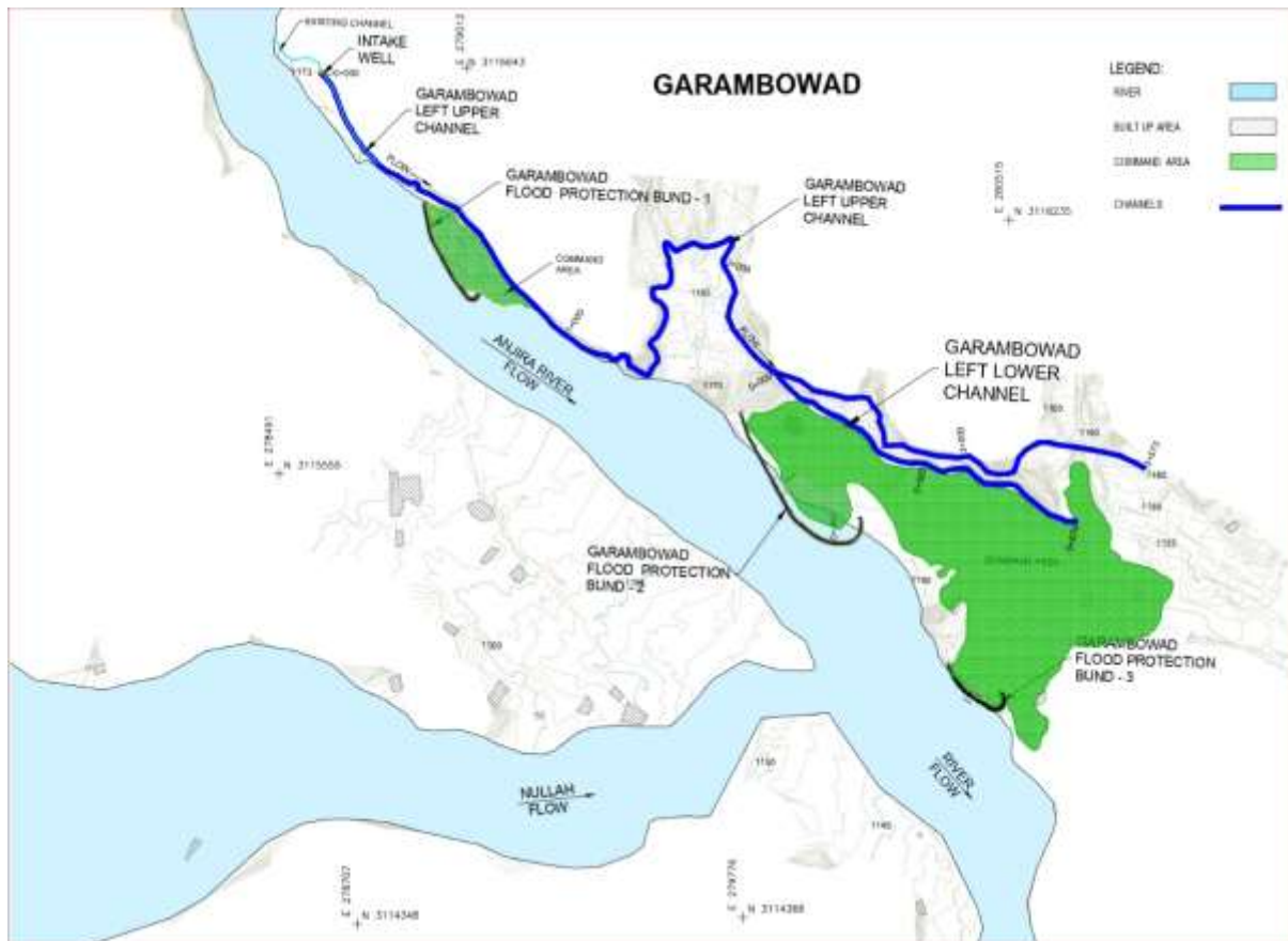
Figure 3-6: Layout of Garambowad Flood Protection Bunds
