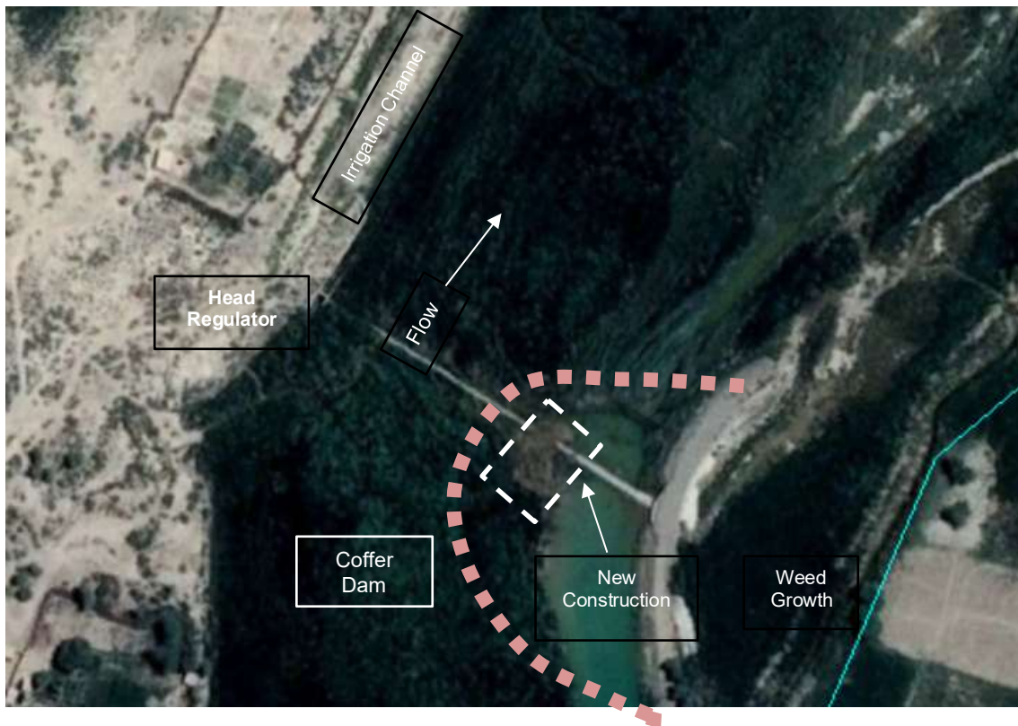
Figure 13: Cofferdam for the construction of damaged weir portion
